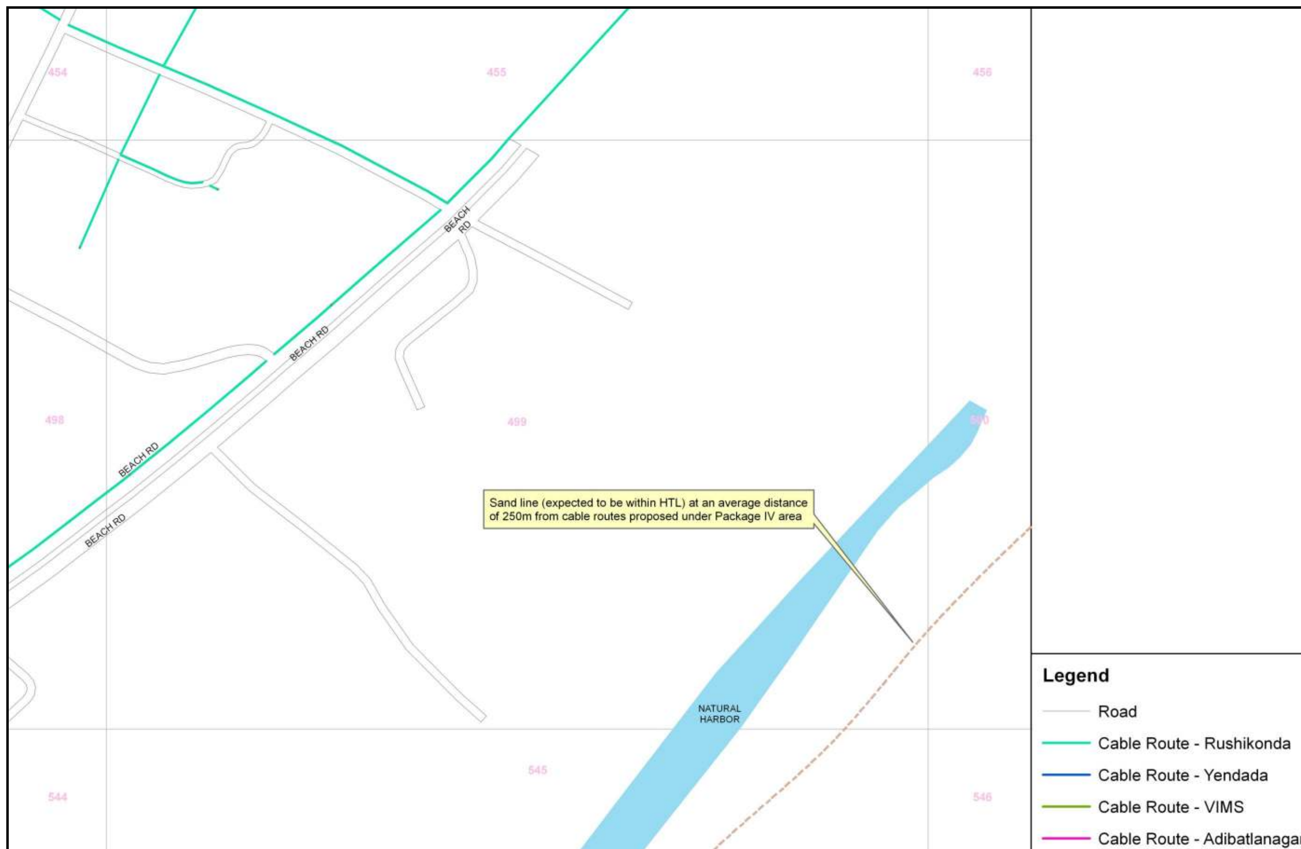
Figure 1n: Distance of the Shore/Sand line (expected to be within HTL) from Cable Routes Proposed under Package 4 Area
