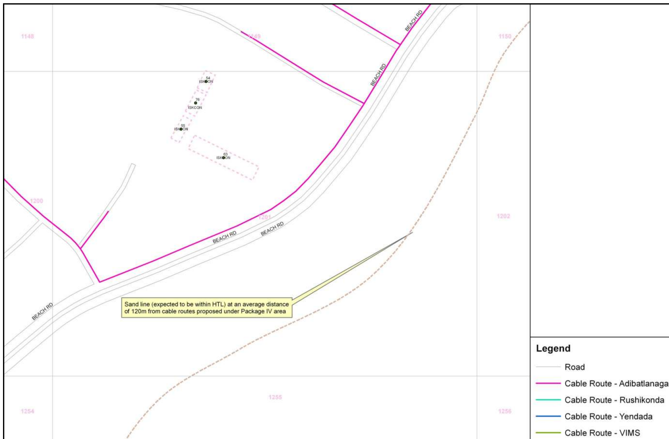
Figure 1h: Distance of the Shore/Sand line (expected to be within HTL) from Cable Routes Proposed under Package 4 Area
